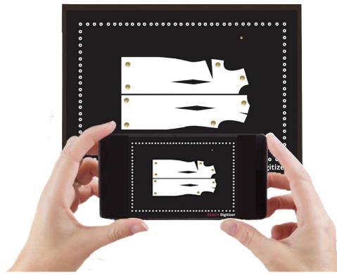
REACH Digitizer enables conversion of physical patterns into digital patterns easily and fast.
